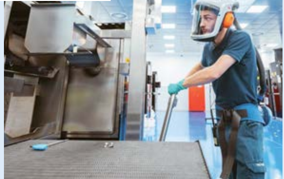
An operator working on a GE Additive Arcam EBM metal 3D printer at Avio Aero's facility in Cameri, Italy.
