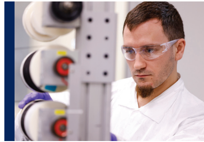
GE Aerospace lab specialist Dakota Martin inspects spools of Ceramic Matrix Composite fiber, a centerpiece of GE Aerospace's 21st century commercial and military engine strategy.
